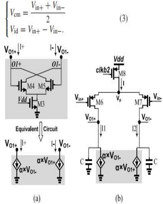
Fig. (a) Equivalent circuit of the cross-coupled part. (b) Simplified circuit diagram of the preamplifier.
