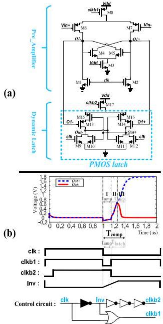
Fig.. (a) Proposed two-stage dynamic. (b) Its typical output waveform and clock signal.
